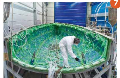
▲ Vacuum infusion underway on a Euphoria 54 hull. Infusion with DSM vinylester resin takes around 2.5 hours
