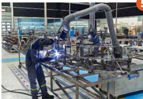
▲ Sirena produces its own stainless steel work, cutting, shaping and welding items then polishing them to a high mirror finish
