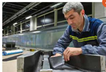
▲ Sirena moulds its own carbon spars. It is one of only a few boatbuilders to offer carbon masts as standard
