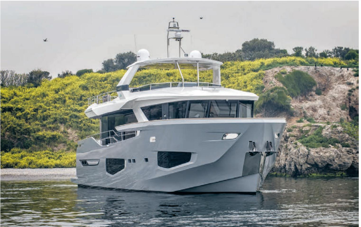
THE NUMARINE XP26, IN DISPLACEMENT VERSION, WILL REACH A MAXIMUM SPEED OF 11.5 KNOTS AND A CRUISING SPEED OF 9 KNOTS. IN ADDITION, IT OFFERS GREATER FUEL AUTONOMY, UP TO 3,500 MILES AT 8 KNOTS. THE FLEXIBILITY OF THE DESIGN CONCEPT IS ANOTHER OF THE GREAT ADVANTAGES OF THE 26XP
